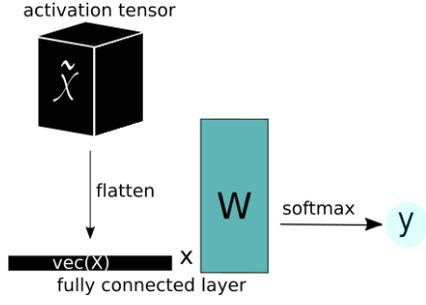
Figure 2: In a traditional deep neural network architecture, the input tensor  $\tilde{\mathcal{X}}$  is flattened and passed on to a fully connected layer, where it is multiplied by a weight matrix  $\tilde{\mathbf{W}}$ .
