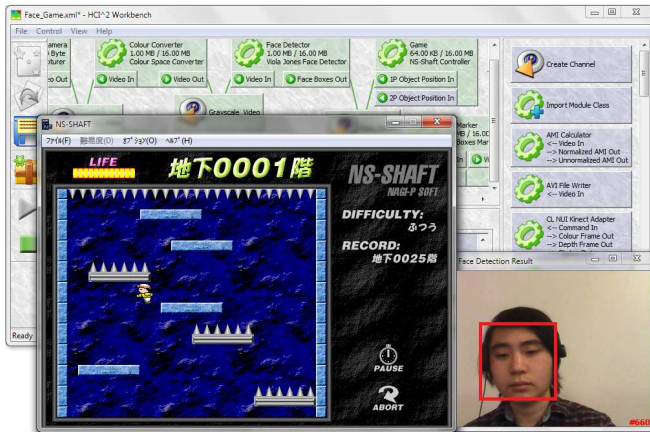
Fig. 11. The CamGame variant using face position.
