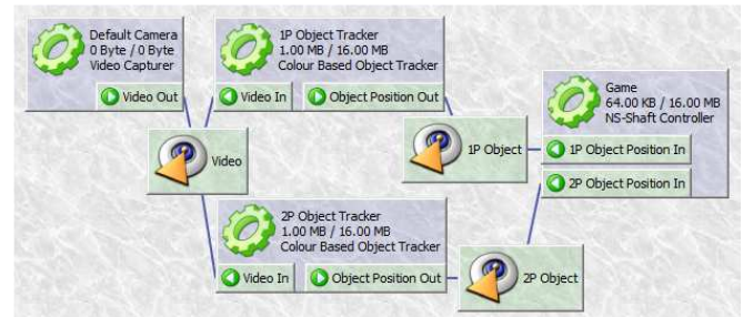
Fig. 9. The baseline CamGame system in a cooperative-mode using a single camera.
