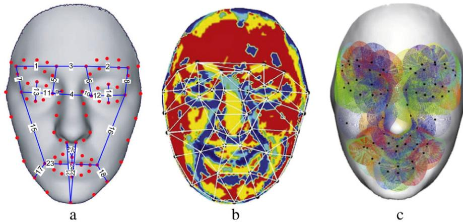
**Fig. 9.** Different features based on the 83 given facial points in the BU-3DFE database. (a) Distance between particular given facial points used in [106,92,107,108]. (b) Distance and curvature features used in [95]. (c) Circular patches around each facial point used in [101,109]. Image (a) taken from [106], (b) taken from [95] (c) taken from [101].
