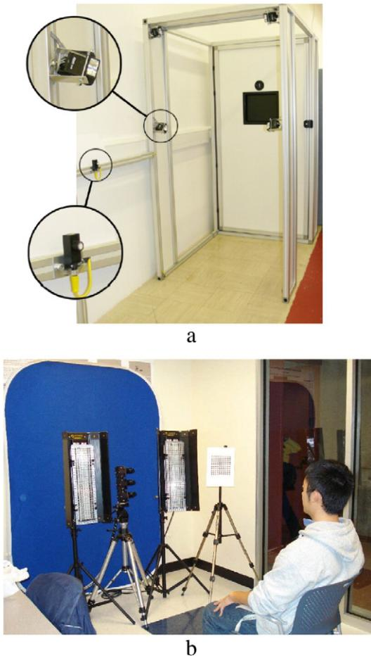
**Fig. 6.** The different setups for two types of stereo acquisition. (a) Photometric stereo acquisition setup. (b) Multi-view stereo acquisition setup.
