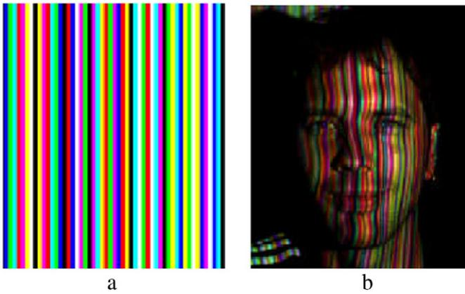
**Fig. 4.** Example of structured light. (a) The light structure used. (b) This light structure projected onto a face. Images taken from [23].
