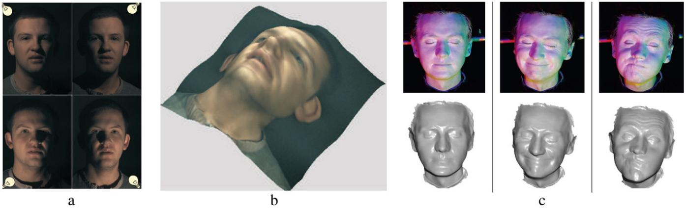
**Fig. 5.** Comparison of the photometric stereo and multispectral photometric stereo. (a) Photometric stereo illumination method. (b) 3D facial data captured by photometric stereo. (c) Multispectral photometric stereo capturing the subject with different coloured light in different direction. Image (c) is taken from [39].
