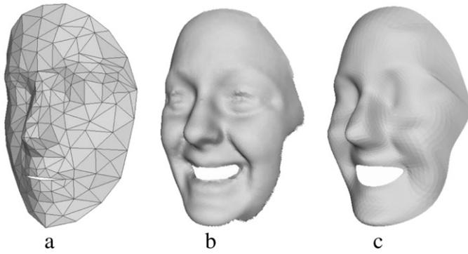
**Fig. 10.** Morphable model fitting in [69,113,114]. (a) The base mesh. (b) The original surface data. (c) The base mesh fitted to the surface. Images taken from [69].
