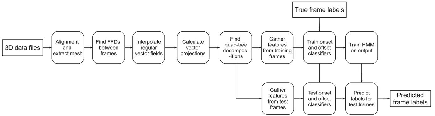
Fig. 1. An overview of the full system including motion caption, feature extraction, classification, and training and testing.
