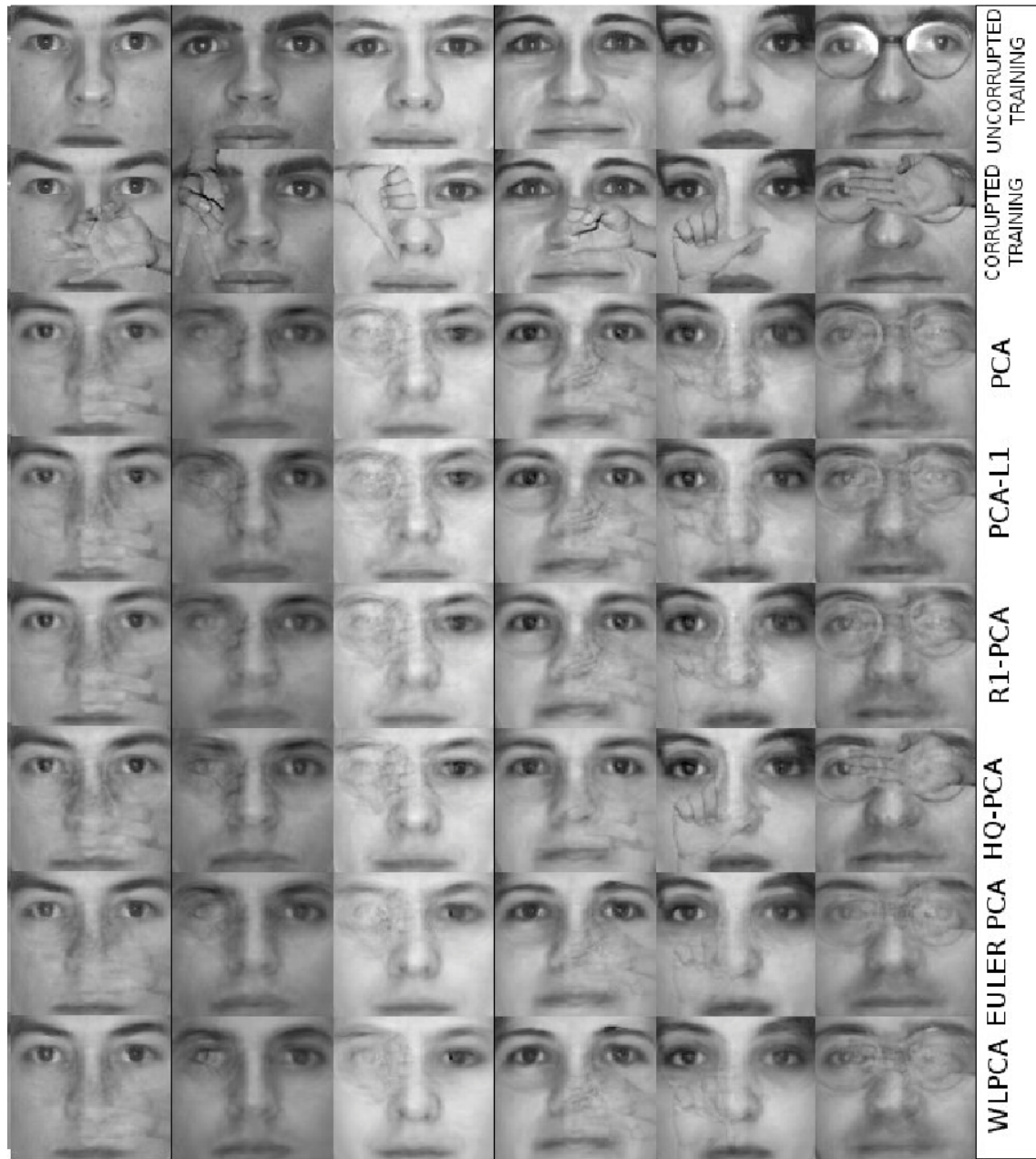
Fig. 6. Reconstruction of PCA, PCA-L1, R1-PCA, HQ-PCA, EULER-PCA and Widely Linear PCA after learning with 50% hand occluded images in AR database.
