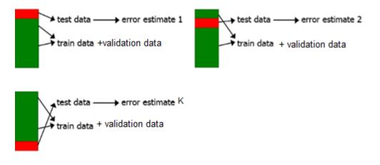
Fig.4: K-fold cross-validation process.
