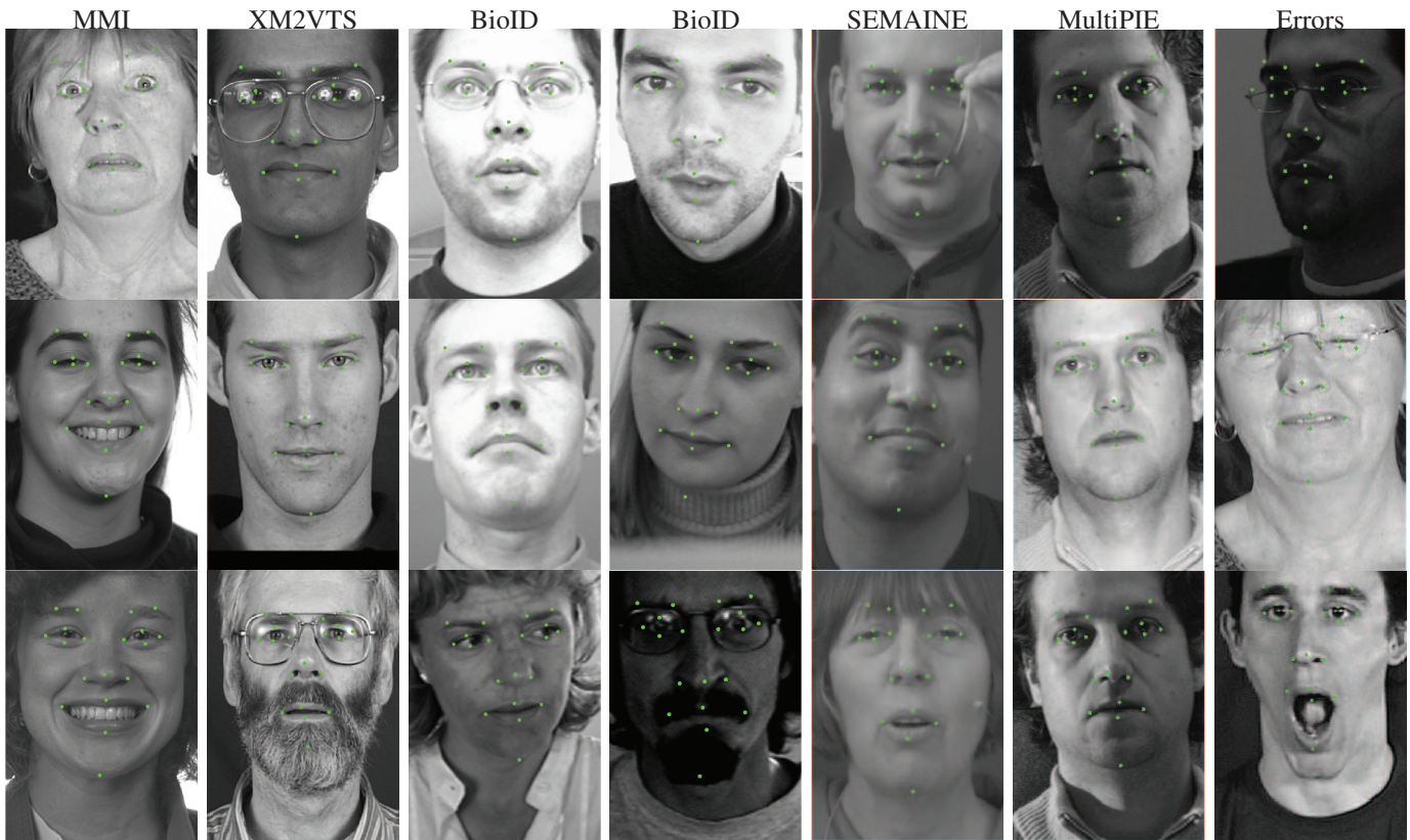
Fig. 6. Results of the point detector on images in the different databases used, and prototypical errors (out of plane rotation, facial hair, and extreme facial expressions). Each column displays examples of the database indicated on its top. The examples of the MultiPIE database show the detection for the first subject of session 3 (first subject of the portion considered here) for frontal and lateral illumination conditions. The errors are 0.067, 0.046 and 0.052 respectively.
