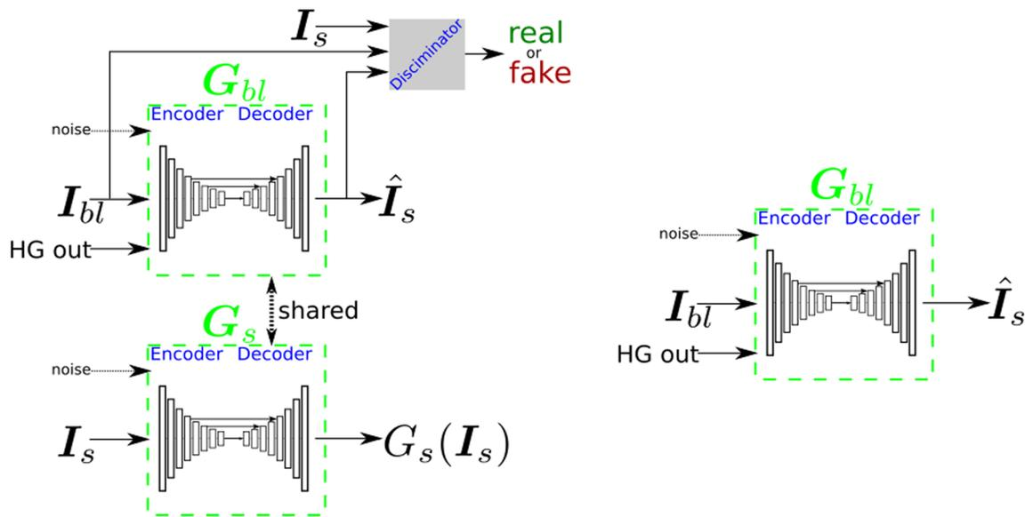
**Fig. 3** Schematic of our cGAN (Sect. 3.2). The training time cGAN is depicted in the left. ‘HG out’ signifies the additional label used as input, i.e. the output of the HG network, while the weight sharing of the
