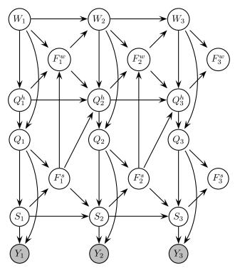
Figure 2.19: A DBN for continuous speech recognition. Note that the observations,  $Y_t$ , the transition probabilities,  $S_t$ , and the termination probabilities,  $F_t^S$ , are conditioned on the phone  $Q_t$ , not the position within the phone HMM  $Q_t^h$ , and not on the word,  $W_t$ .
