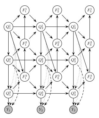
Figure 2.14: A 3-level HHMM represented as a DBN.  $Q_t^d$  is the state at time t, level d;  $F_t^d=1$  if the HMM at level d has finished (entered its exit state), otherwise  $F_t^d=0$ . Shaded nodes are observed; the remaining nodes are hidden. In some applications, the dotted arcs from  $Q^1$  and the dashed arcs from  $Q^2$  may be omitted.
