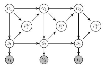
Figure 2.29: A 1-level AHMM.  $F_t^G$  turns on if state  $S_t$  statisfies goal  $G_t$ ; this causes a new goal to be chosen. However, the new state may depend on the old state; hence there is no arc from  $F_{t-1}^G$  to  $S_t$  to "reset" the submodel.
