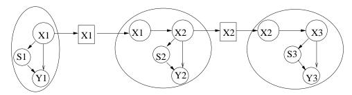
Figure 3.7: The DAGs for an HMM with mixture of Gaussians output, glued together by their interface nodes,  $X_t$ . The non-interface is  $N_t = (S_t, Y_t)$ .
