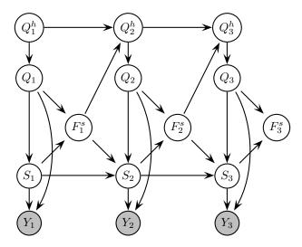
Figure 2.17: A DBN for modelling the pronunciation of a single word.  $Q^h$  is the state (position) in the word HMM; Q is the phone; S is the state (position) within the phone HMM, i.e., the subphone; Y is the acoustic vector.  $F^s$  is a binary indicator variable that turns on when the phone HMM has finished.
