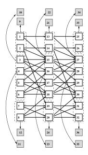
Figure 4.1: The water DBN, designed to monitor a waste water treatement plant. This model is originally from [JKOP89], and was modified by [BK98b] to include (discrete) evidence nodes. The dotted arcs group together nodes that will be used in the BK approximation: see Section 4.2.1. Nodes are numbered in topological order, as required by BNT.
