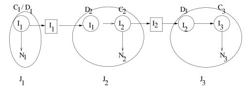
Figure 3.6: A schematic illustration of how to join the junction trees for each  $1\frac{1}{2}$ -slice DBN.  $I_t$  are the interface nodes for slice t,  $N_t$  are the non-interface nodes.  $D_t$  is the clique in  $J_t$  containing  $I_{t-1}$ .  $C_t$  is the clique in  $J_t$  containing  $I_t$ . The square box represents a separator, whose domain is  $I_t$ .
