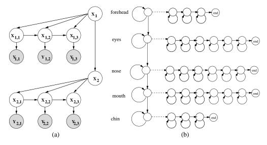
Figure 2.24: An embedded HMM for face recognition represented (a) as a DBN and (b) as the state transition diagram of an HHMM (dotted arcs represent calling a sub-HMM). We assume there are 2 rows and 3 columns in the image, which is clear from the DBN representation, but not from the HHMM representation. The number of states in each sub-model can be different, which is clear from the HHMM but not the DBN. The DBN in (a) is just a rotated version of the one in Figure 2.23.
