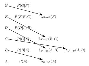
Figure B.2: Variable elimination applied to Figure B.1 using the ordering A, B, C, D, F, G. The arrow from F to C means we compute the "message"  $\lambda_{F\to C}(B,C)=\sum_F P(F|C,B)\lambda_{G\to F}(F)$  and send it to C's "bucket", etc.
