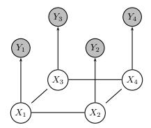
Figure A.4: A pairwise MRF defined on a lattice. Each hidden variable  $X_i$  has its own "private" observed child  $Y_i$ . Technically, this is a chain graph since the arcs from  $X_i$  to  $Y_i$  are directed.
