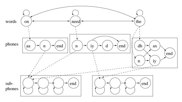
Figure 2.20: An example HHMM for an ASR system which can recognize 3 words (adapted from [JM00]). The phone models (bottom level) are shared (tied) amongst different words; only some of them are shown.
