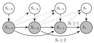
Figure 2.8: A mixed-memory Markov model. The dashed arc from  $S_t$  to  $X_t$  means  $S_t$  is a switching parent: it is used to decide which of the other parents to use, either  $X_{t-1}$  or  $X_{t-2}$  or both. The conditions under which each arc is active are shown for the  $X_t$  node only, to reduce clutter. The dotted arcs from  $X_{t-1}$  and  $X_{t-2}$  to  $S_t$  are optional. See text for details. Based on Figure 15 of [Bil01].
