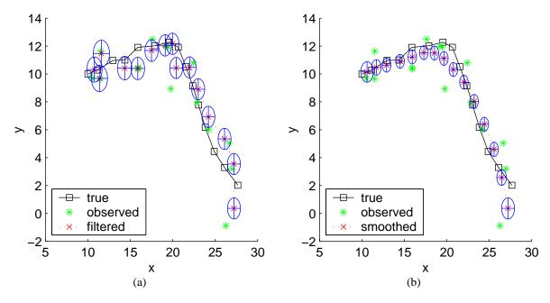
Figure 1.3: Results of inference for the the tracking problem in Section 1.3.1. (a) Filtering. (b) Smoothing. Boxes represent the true position, stars represent the observed position, crosses represented the estimated (mean) position, ellipses represent the uncertainty (covariance) in the position estimate. Notice that the smoothed covariances are smaller than the filtered covariances, except at t=T, as expected.
