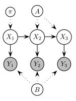
Figure 2.2: An HMM in which we explicitly represent the parameters (nodes with outgoing dotted arcs) and the fact that they are tied across time-slices. The parameters are  $P(X_1 = i) = \pi(i)$ ,  $P(X_t = j | X_{t-1} = i) = A(i, j)$ , and  $P(Y_t = j | X_t = i) = B(i, j)$ . If the CPD for Y is a Gaussian, we would replace the B node with the mean and covariance parameters.
