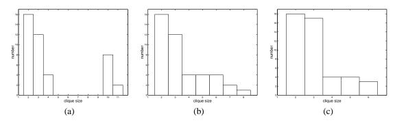
Figure 4.3: Clique size distribution for different levels of BK approximation applied to the BATnet (Figure 4.2). The cliques of size 2 are due to the observed leaves. (a) Exact: the interface is  $\{7, 14, 16, 17, 19, 20, 21, 23, 25, 27\}$ . (b) Partial approximation: the interface sets are  $\{7, 14, 16, 17, 19\}$  and  $\{20, 21, 23, 25, 27\}$ , as in Figure 4.2. (c) Fully factorized approximation: the interface sets are the singletons.
