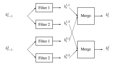
Figure 4.14: The GPB2 algorithm for the case of a binary switch.  $b_{t-1}^i = P(X_{t-1}, S_{t-1} = i | y_{1:t-1})$  is the prior,  $b_t^{i,j} = P(X_t, S_{t-1} = i, S_t = y | y_{1:t})$ , and  $b_t^j = P(X_t S_t = y | y_{1:t})$  is the approximate posterior. The filter box implements the Kalman filter equations (see Section 3.6.1). The merge box implements the weak marginalization/moment matching equations (see Section B.5.2).
