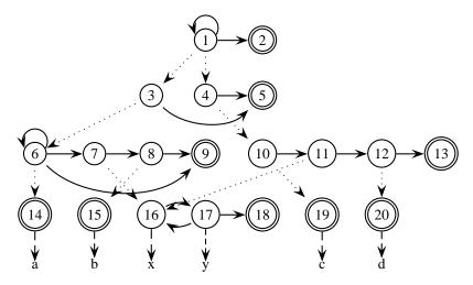
Figure 2.15: State transition diagram of the HHMM in Figure 2.12, except all production states are at the leaves.
