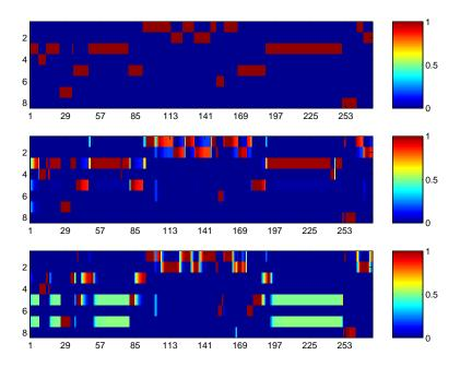
Figure 6.10: Inferring goals using three different methods. Rows represent states (goal locations), columns represent time. Shading represents  $P(G_t|y_{1:t})$ . First line: ground truth. Second line: using the learned goal transition matrix. Third line: using a uniform goal transition matrix.
