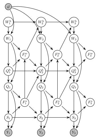
Figure 2.21: A DBN for training a continuous speech recognition system from a known word sequence  $\vec{w}$ . In practice, the  $\vec{w}$  node can be absorbed into the CPDs for W. Also, if the mapping from words to phones is fixed, we can also compile out  $W^h$ , W, and  $F^W$ , resulting in the much simpler model shown in Figure 2.17 (or Figure 2.18 if we don't use subphones).
