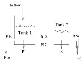
Figure 2.33: The two-tank system. The goal is to infer when pipes are blocked or have burst, or sensors have broken, from (noisy) observations of the flow out of tank 1, F1o, out of tank 2, F2o, or between tanks 1 and 2, F12. R1o is a hidden variable representing the resistance of the pipe out of tank 1, P1 is a hidden variable representing the pressure in tank 1, etc. From Figure 11 of [KL01].
