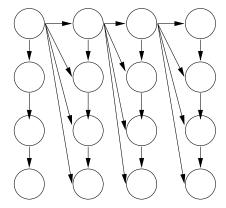
Figure 3.5: The "cascade" DBN, from Figure 2 of [Dar01]. This graph has a treewidth of 2.
