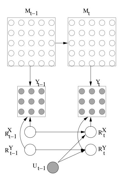
Figure 5.7: The DBN used in the map-learning problem. M represents the map, R the robot's location, Y the observation, and U the input (control). There is one arc from each (i,j) cell of  $M_t$  to  $Y_t$ . Similarly, each (i,j) cell of  $M_t$  connects to the corresponding (i,j) cell in  $M_{t+1}$ .  $P(Y_t|M_t,L_t)$  is a multiplexer CPD, i.e.,  $P(Y_t|M_t,L_t=j)=f(Y_t,M_t(j))$ .
