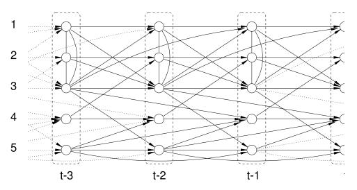
Figure 2.30: A VAR(2) process represented as a graphical model. From [DE00]. The link from  $X_{t-3}^3 \to X_{t-1}^4$  exists because  $A_2(4,3) = \frac{1}{5} > 0$ .
