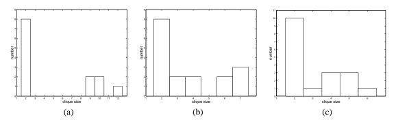
Figure 4.4: Clique size distribution for different levels of BK approximation applied to the water DBN (Figure 4.1). The cliques of size 2 are due to the observed leaves. (a) Exact: the interface is  $\{1, \ldots, 8\}$ . (b) Partial approximation: the interface sets are  $\{1, 2\}$ ,  $\{3, 4, 5, 6\}$  and  $\{7, 8\}$ , as in Figure 4.1. (c) Fully factorized approximation: the interface sets are the singletons.
