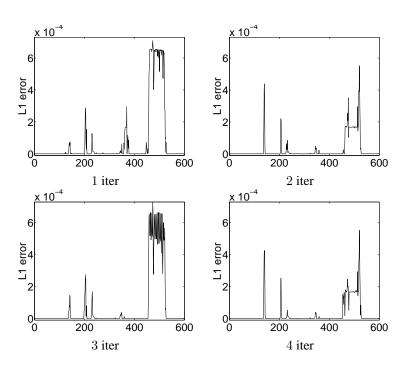
Figure 4.7:  $L_1$  error on marginal posteriors vs. timeslice after iterations 1–4 of undamped LBP applied to the traffic CHMM. The  $L_1$  error oscillates with a period of 2 (as seen by the similarity between the graphs for iterations 1/3 and 2/4); this implies that the underlying marginals are oscillating with the same period.
