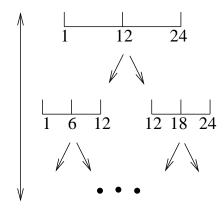
Figure 3.20: The basic idea behind the Island algorithm, with T = 24, C = 1. At the top level, we call Island  $(f_0, b_{25}, y_{1:24})$ , which computes  $b_1$ ,  $b_{12}$  and  $b_{24}$ .  $(f_0$  and  $b_{25}$  are dummy boundary conditions used at the top level.) Then we call Island  $(f_1, b_{12}, y_{2:11})$ , followed by Island  $(f_{12}, b_{24}, y_{13:23})$ .
