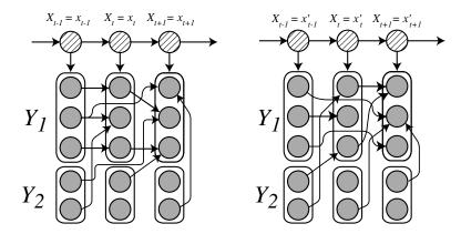
Figure 2.6: A buried Markov model. Depending on the value of the hidden variables,  $X_t$ , the effective graph structure between the components of the observed variables,  $Y_t$ , can change. Two different instantiations are shown. Thanks to Jeff Bilmes for this figure.
