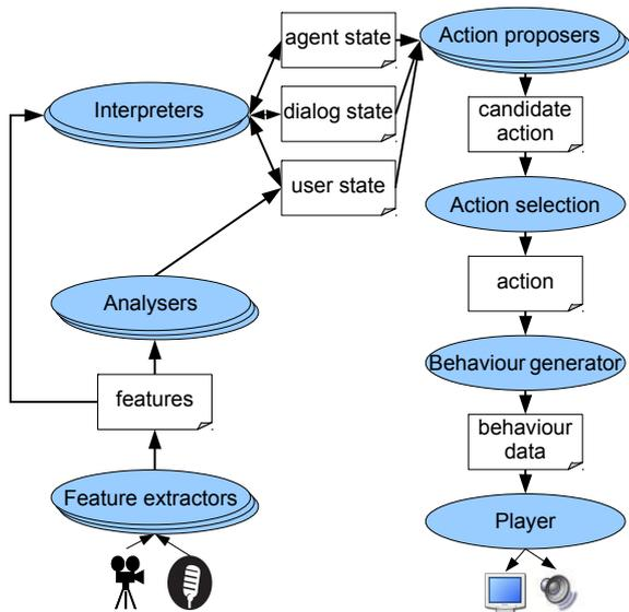
Fig. 1: Conceptual architecture of the SAL system
