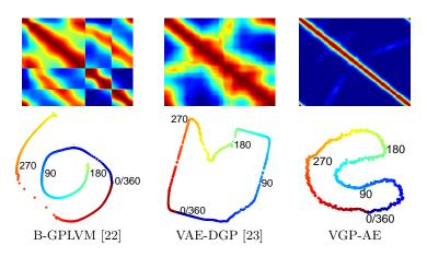
Fig. 2. Recovering the structure of a rotated '1' from MNIST. The learned kernel matrices (upper row) and 2D manifolds (lower row) obtained from B-GPLVM (left), VAE-DGP (middle) and the proposed VGP-AE (right), initialized from the same random instance.
