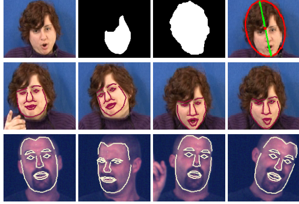
Fig. 1: AAM fitting initialization and result. Top: Initial image, skin masks for width and rotation estimation, similarity rotation via ellipsis. Middle, Bottom: AAM fitting result on GSL and BU.
