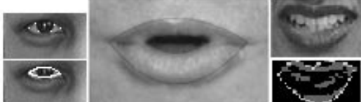
Fig. 4. Curve fitting on eye micro-features, mouth template matching, fitting three 2 nd degree parabolas to the mouth
