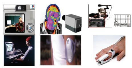
Figure 3: Examples of sensors used in multimodal affective data acquisition: (a) camera for visible imagery, (b) microphone(s) for audio recording, (c) infrared camera for thermal infrared (IR) imagery, (d) body media sense wear for physiological signal recording, (e) pulse wave signal recorder clipped on the finger, and (f) electroencephalogram (EEG) for brain/scalp signals recording and measurement.
