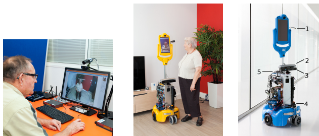
Fig. 1: Left, middle: A user of the TERESA system can remotely interact with others in an elderly day centre. Right: The TERESA telepresence robot. Its most relevant sensors are labeled: 1 – Dalsa Genie TM HM1400; 2 – VoiceTracker TM II; 3 – Microsoft Kinect TM ; 4 – 2x Hokuyo TM UST-10LX; 5 – XSens TM MTi-30 AHRS.
