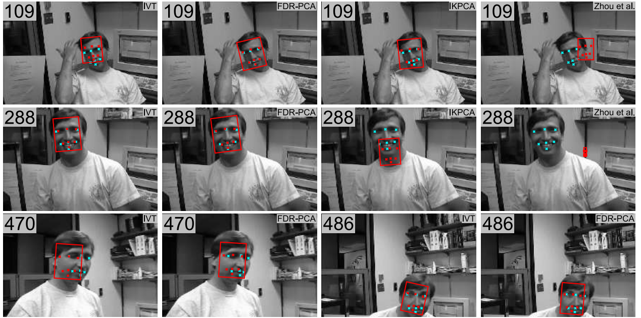
Fig. 3. Tracking results of the different schemes for the Dudek video sequence. The third and fourth column (first two rows) show Zhou et al. [3] and IKPCA – both trackers lose the object. IVT and the proposed tracker is shown in the first and second column (first two rows) respectively. The last row show two examples of some late frames for the proposed and the IVT tracker (the other tested tracks have already lost the face). The ground truth is indicated by cyan-colored points.
