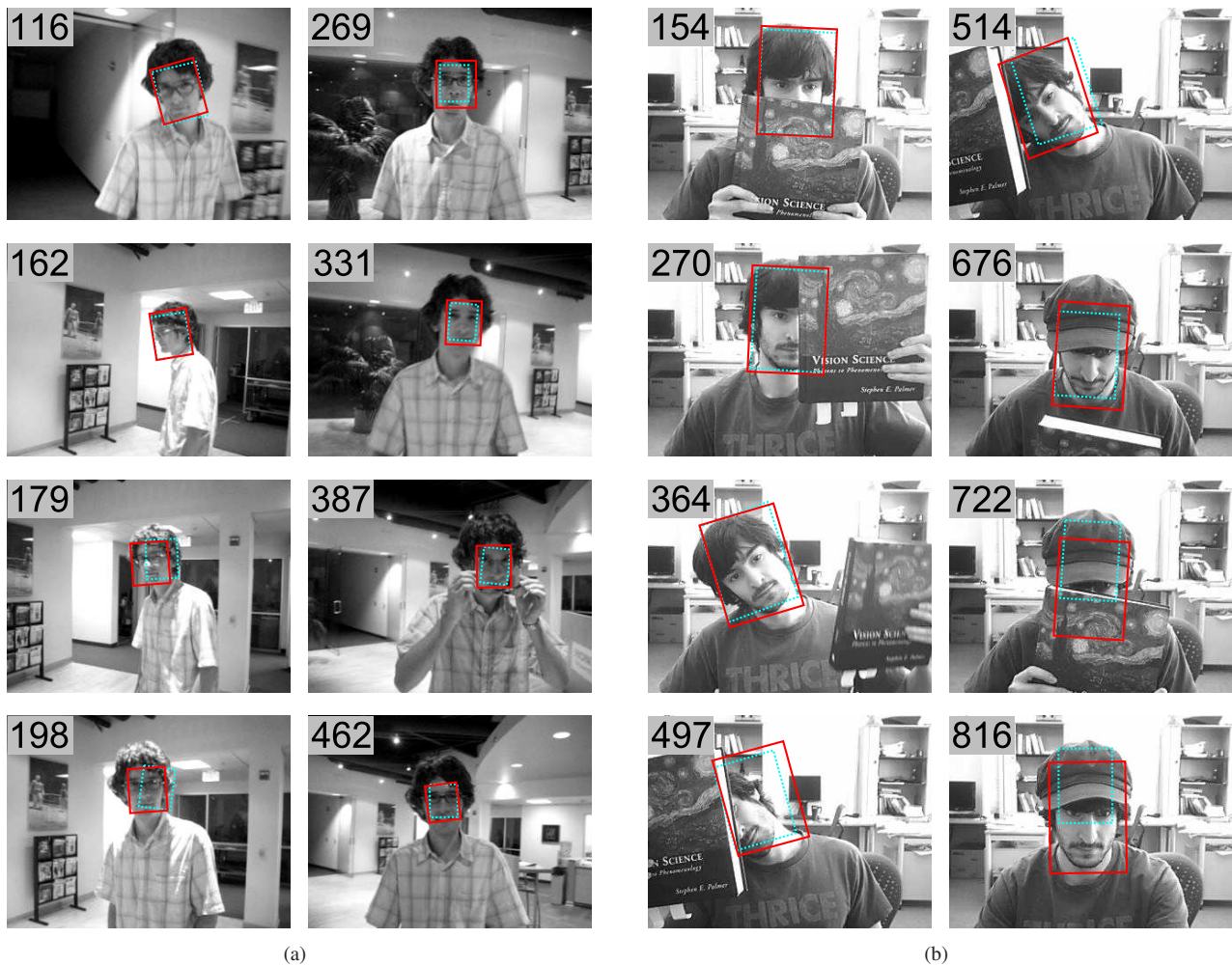
Fig. 7. The results of the proposed tracker (in solid red) compared to the IVT of Ross et al. [9] (in dotted cyan) on different video sequences.
