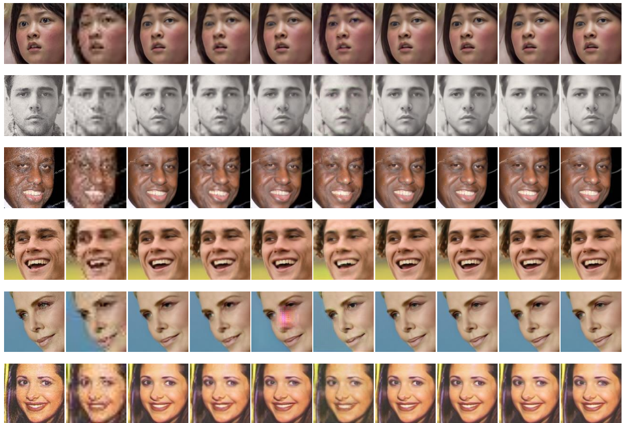
Fig. 9. Visual results of BI models ( \times 4 ) on the EDFace-Celeb-1M dataset. From left to right: HR, results of bicubic, DICNet, DICGAN, WaveletSR, HiFaceGAN, EDSR, RDN, RCAN and HAN. "BI" means the bicubic interpolation.
