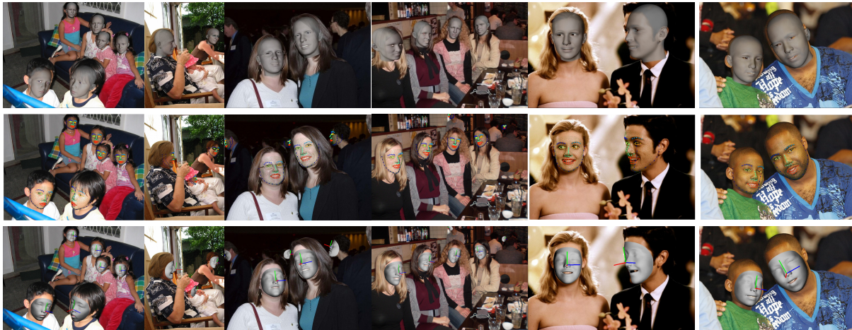
Figure 10. Testing results of RetinaFace (ResNet-50, \mathcal{L}_{5pts+mesh} ) compared to MFN [6] (first row). We show both the predicted 1k 3D vertices (Second row) and the 3D meshes rendered by the Vulkan toolkit (Third row). Please zoom in to check the missing faces (Column 2-4) and obvious mis-alignment (Column 5-6) by MFN.
