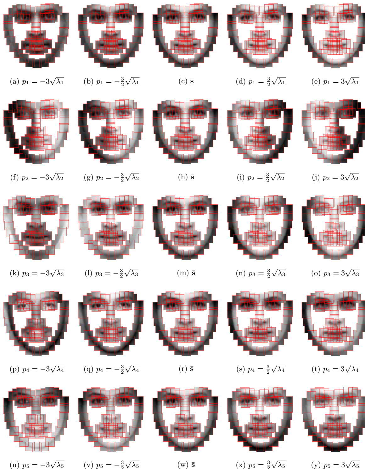
Figure 3.6: Exemplar instances of a part-based statistical appearance model trained on the images of LFPW trainset. Each row shows the variations covered by the first five principal components, where \lambda_i is the eigenvalue that corresponds to the i -th eigenvector.
