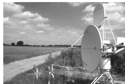
Figure 2. Scanning harmonic radar equipment
