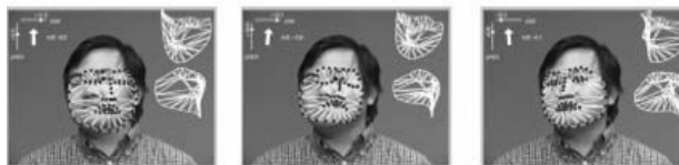
Figure 2. An example of fitting a 2D+3D AAM to a single image. Shown are the initial fit, intermediate result, and final result after the algorithm has converged. The 3D shape estimate (white) is projected onto the original image and also from two novel viewpoints (top right). Estimates of 3D pose (top left) and 2D shape (blue dots) are displayed as well. Estimated head orientation (pitch, roll, and yaw) is shown in the top left-hand corner of each image. From [25]
