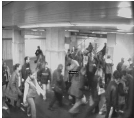
Figure 5. Detection of stationary object (a suitcase to the right of the central pillar).
