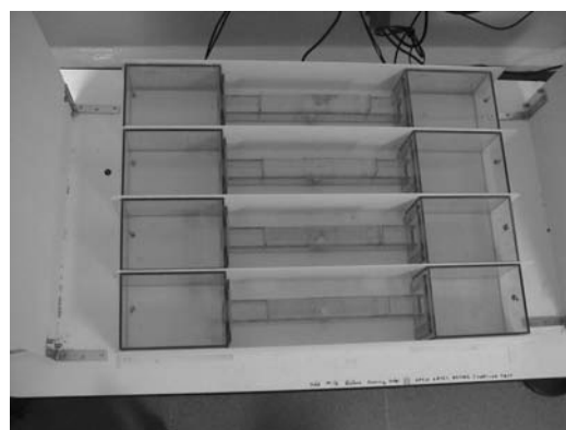
Figure 4. DSR test apparatus: the experimental set-up as viewed by the overhead video-camera. A unit of the apparatus consists of two plexiglass chambers connected by a passage having a small feeder dish with milk in the center from which only one rat can drink sweetened milk at a time. Four units are placed in parallel. The time spent at the feeder is scored for each of eight rats (four pairs) during one 5-minute experimental session.
