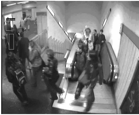
Figure 4. Maintaining detection of lingering people during occlusion (person on left hand side by the wall poster).
