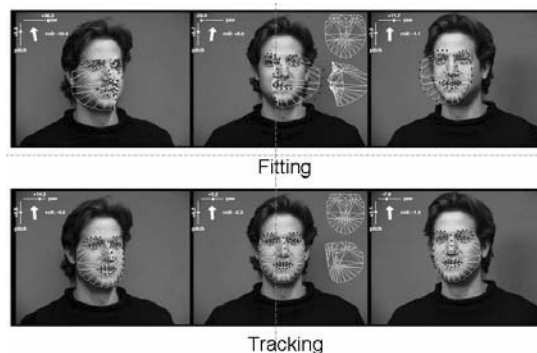
Figure 4. An example of multi-view 3D AAM fitting. Each image is overlaid with the corresponding 2D shape for that image in blue dots. The head pose is displayed in the top left of each image as pitch, roll, and yaw. The single 3D shape is displayed in the top right of the center image. This 3D shape is also overlaid in each image as a white mesh. From [15].
