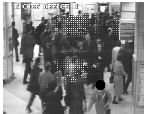
Figure 3. Automatic identification of congestion (dense non-moving area), denoted by array of white dots.
