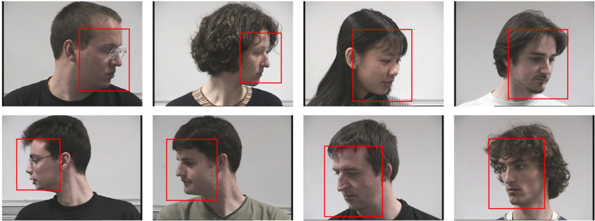
Fig. 6. MVFD with CDPM on HPID. We tested the performance of our 4 * (Roots + 6Parts) CDPM on images from the HPID databases. These images are annotated with pan and tilt head rotations of \pm 90^\circ , \pm 75^\circ , \pm 60^\circ and \pm 45^\circ .
