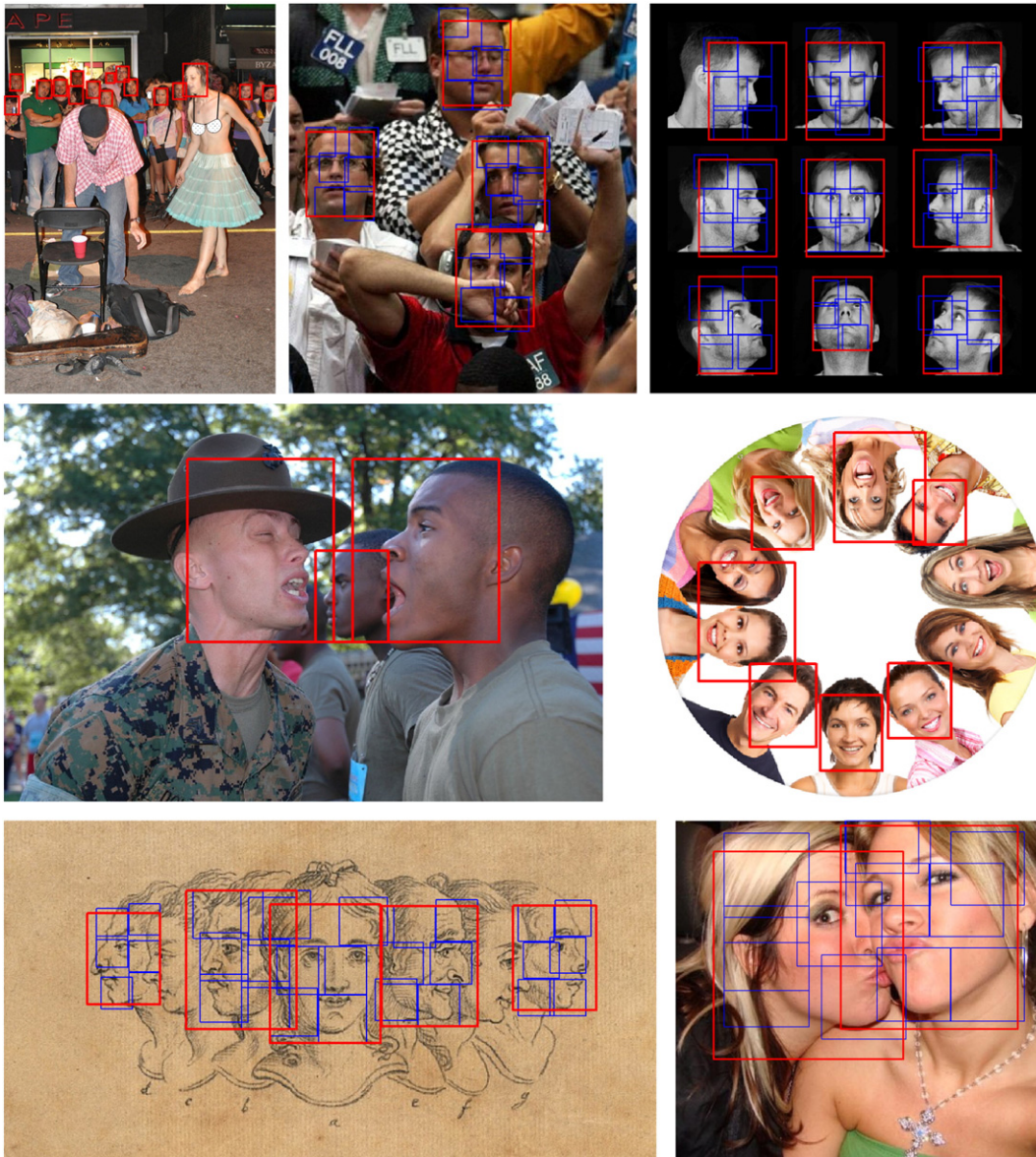
Fig. 5. Multi-view face detection with CDPM. These examples were obtained with the 4 * (Roots + 6Parts) CDPM on images from the Fddb and AFLW databases. Red bounding boxes determine the best location for the root filters whereas blue boxes are used for the part filters detections.
