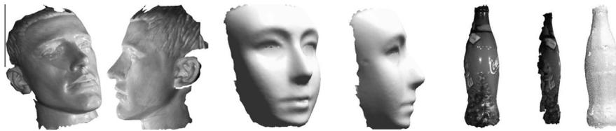
Fig. 25. 3D surfaces obtained using the 3dMD imaging system.
