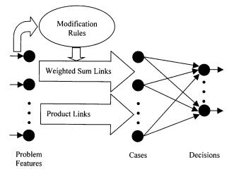
Fig. 3. A layered neural network model for CBR.
