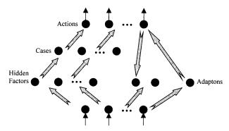
Fig. 4. A layered neural network model with hybrid connection for CBR.
