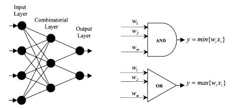
Fig. 5. The structure of the Combinational Neural Model (CNM) and node characters.
