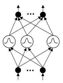
Fig. 1. The topology of a RBF network.
